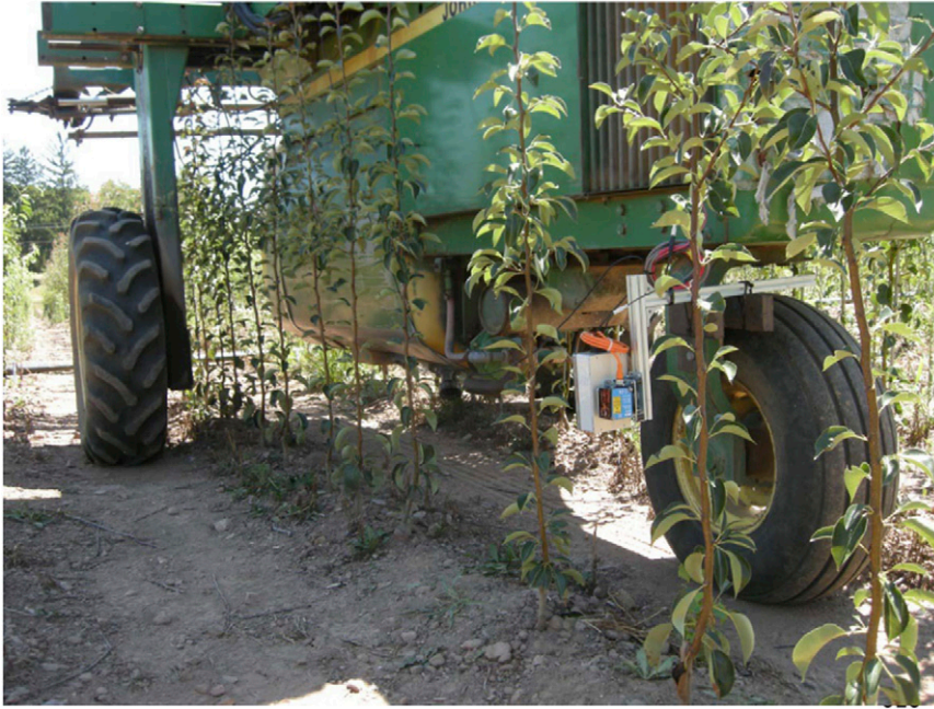
Fig. 3. On-the-Fly counter and caliper. Sensors were designed by Carnegie Mellon University (Pittsburgh, PA) engineers to count trees in a nursery field and to determine the diameter of the trunks. The sensor shown here is used to take an inventory of trees before harvest.
