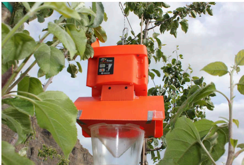
Fig. 2. Electronic insect trap designed by Spensa Technologies (West Lafayette, IN). Like current traps, it uses pheromones to attract target insects. Its novelties are a high-voltage coil to stun insects entering the trap, bio-impedance sensors to count insects automatically as they fall into the trap, a wireless connection to send pest information directly to a server on the farm, and handheld, web-based software to manage the entire system.
